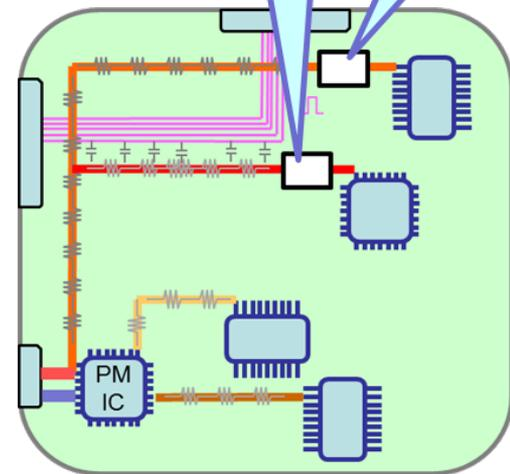
In long wiring portions or for circuits susceptible to noise, local power supply ICs are arranged near the LSIs.
