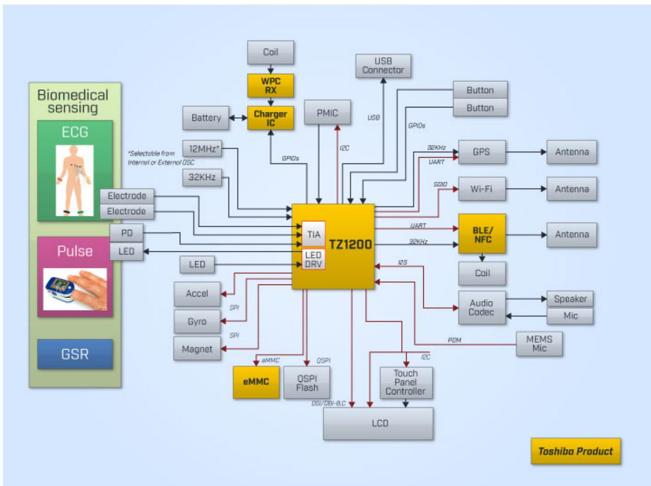
Figure 8: The TZ1200 forms the heart of many sophisticated wearable devices
