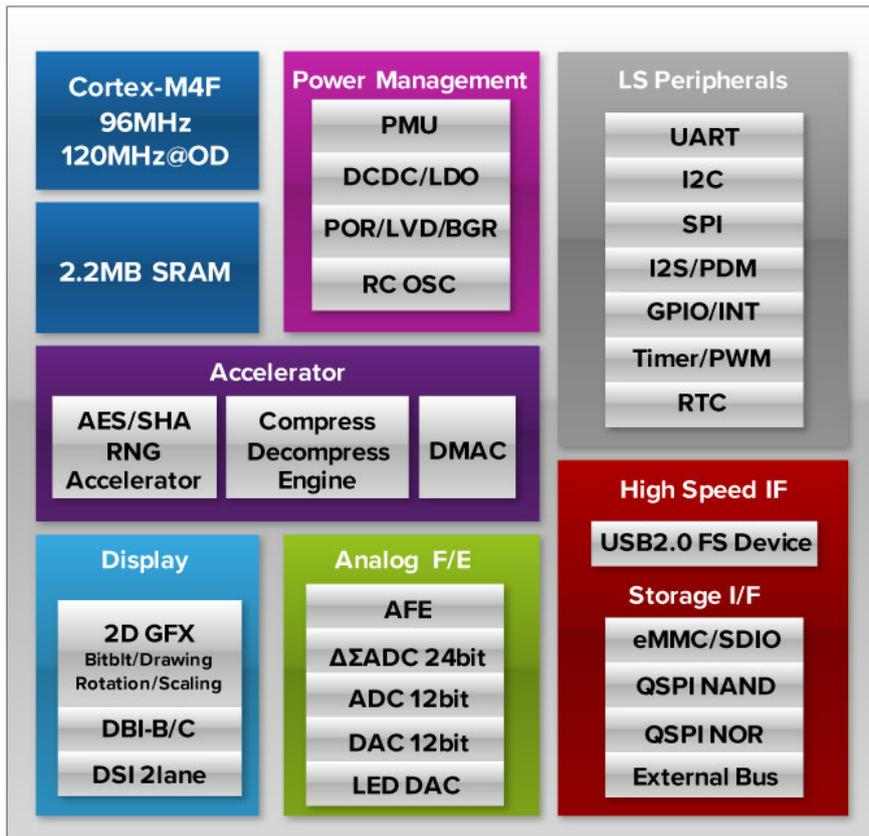
Figure 1: TZ1200 highly integrated solution for wearable devices
