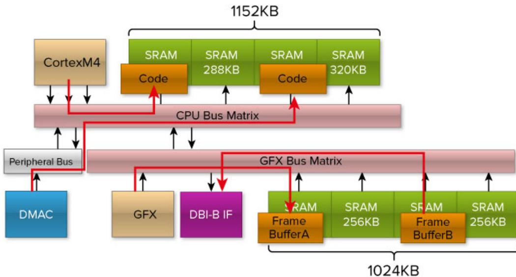
Figure 7: The TZ1200 features separate bus matrices for CPU and graphics operations
