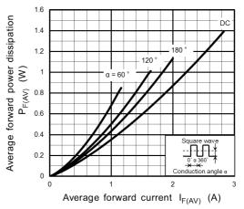
Fig. 10.2 P<sub>F(AV)</sub> - I<sub>F(AV)</sub>
