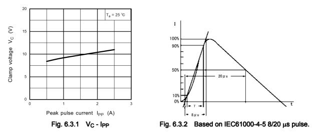
Note: The above characteristics curves are presented for reference only and not guaranteed by production test, unless otherwise noted.
