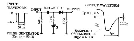
Fig.1 Reverse Recovery Time (t<sub>rr</sub>) Test Circuit
