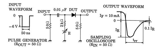
Fig.1 Reverse Recovery Time (t<sub>rr</sub>) Test Circuit
