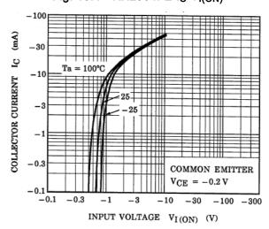
Fig. 10.6 RN2906FE I<sub>C</sub>-V<sub>I(ON)</sub>
