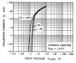
Fig. 10.1 RN2901FE I<sub>C</sub>-V<sub>I(ON)</sub>
