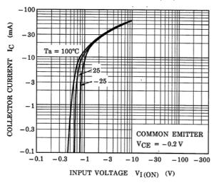
Fig. 10.5 RN2905FE I<sub>C</sub>-V<sub>I(ON)</sub>
