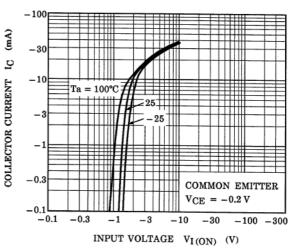
Fig. 10.2 RN2902FE I<sub>C</sub>-V<sub>I(ON)</sub>
