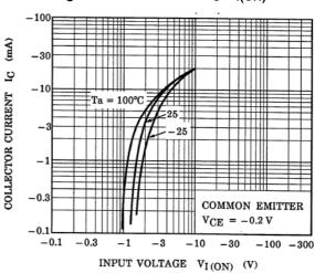
Fig. 10.4 RN2904FE I<sub>C</sub>-V<sub>I(ON)</sub>
