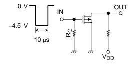
Fig. 5.3.1 Switching Time Test Circuit
