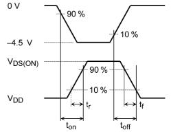
Fig. 5.3.2 Input Waveform/Output Waveform
