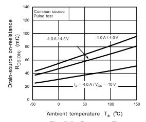
Fig. 7.5 R<sub>DS(ON)</sub> - T<sub>a</sub>
