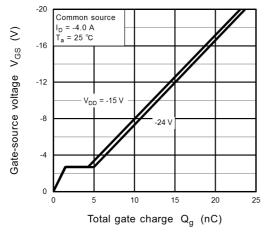
Fig. 7.9 Dynamic Input Characteristics
