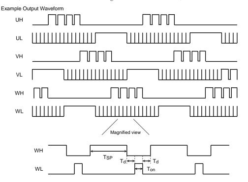
$T_{SP}$ : Variable depending on the VSP (the figure above being applicable when VSP = 5.4 V (typ.));  $T_{ON} = 18/f_{OSC}$ ;  $T_{ON} = 18/f_{OSC}$
