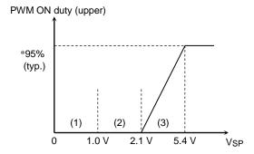
\*: The maximum ON duty is Ton = 95% (typ.) when VSP = 5.4 V (typ.). Example: If fosc = 5 MHz, then ON time = 48  $\mu s$  (typ.) (fc = 19.8 kHz) If fosc = 4 MHz, then ON time = 60  $\mu s$  (typ.) (fc = 15.9 kHz)
