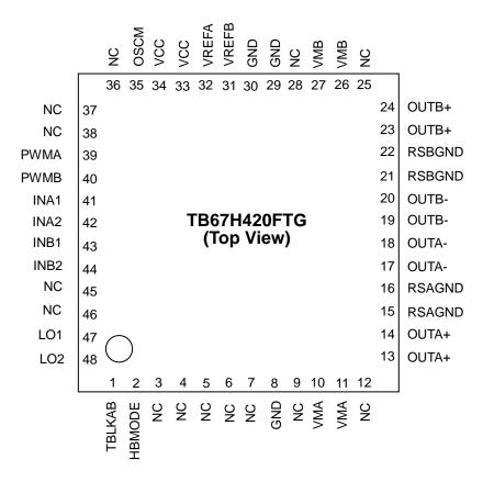
Note: Please solder the corner pad and the bottom thermal pad of the QFN package, to the GND pattern of the PCB. Note: Pin names in the above figure are in the state when HBMODE is low level.
