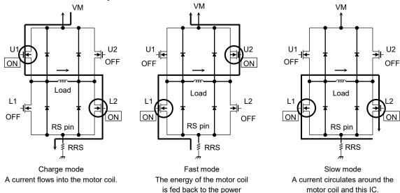
**Operation Function of Output Transistor**
