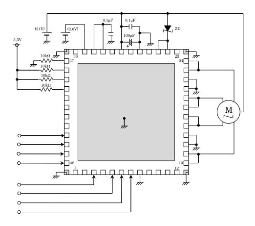
Please mount the four corner pins of the QFN package and the exposed pad to the GND area of the PCB.
