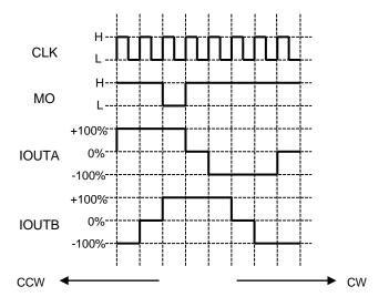
Waveform of MO output: State of pull-up.
