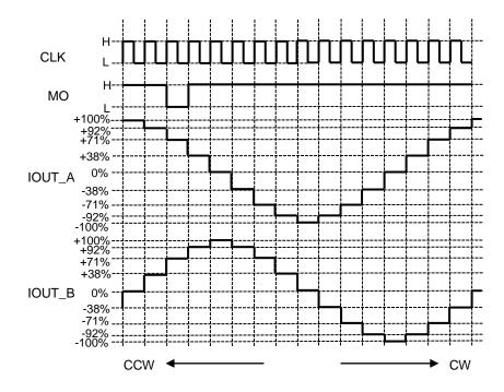
Waveform of MO output: State of pull-up.
