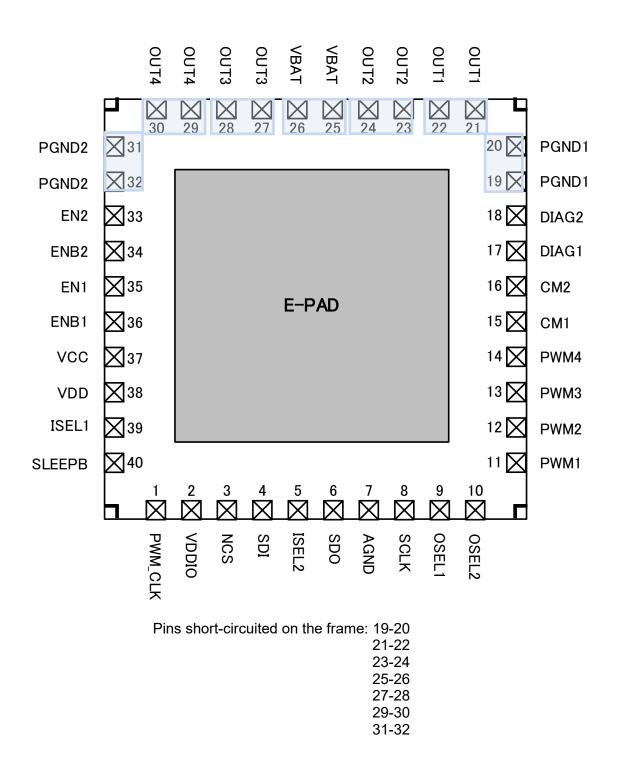
Figure 5.1. Pin assignment
