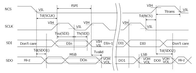
Figure 10.4. SPI communication timing chart
