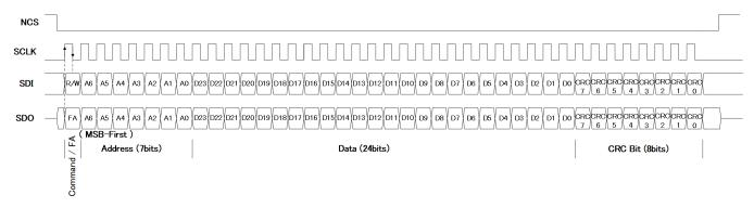
Figure 7.26 SPI communication format
