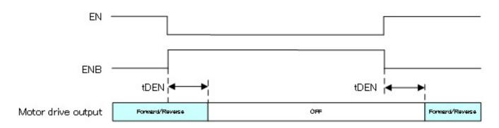
Figure 7.1. EN/ENB signals and motor drive output
