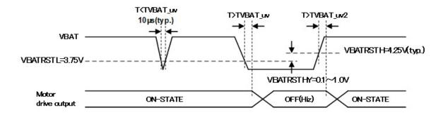
Figure 7.36 VBAT under-voltage detection timing chart 1
