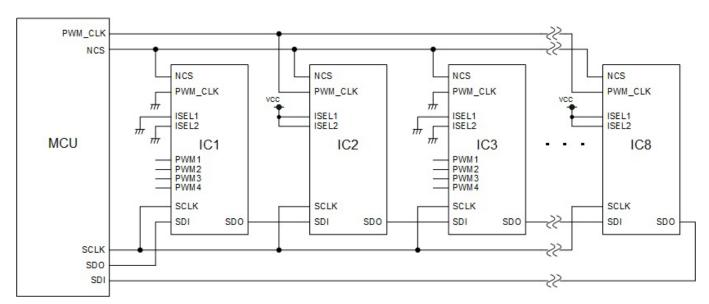
Figure 7.34 Example daisy-chain connection containing both PWM input motor drive and SPI motor drive ICs
