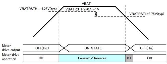
Figure 7.35 VBAT under-voltage detection threshold characteristics
