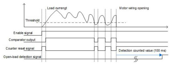
Figure 7.23 Open-load detection during operation: operation waveform
