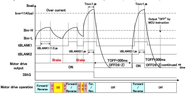
Figure 7.42 Over-current detection operation for short-circuit to power supply or ground, and short-circuited load: timing chart 1
