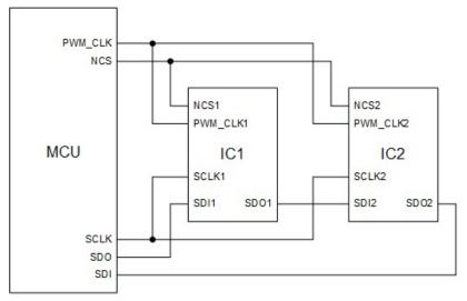
Figure 7.29 Example SPI daisy-chain connection for two ICs
