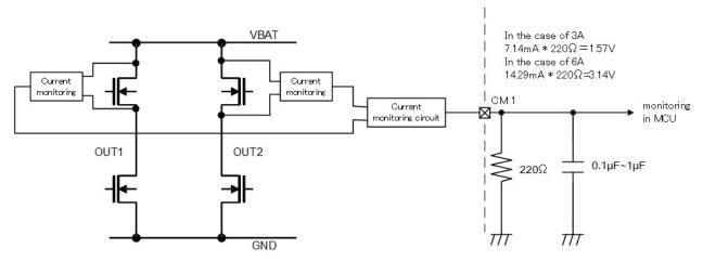
Figure 7.18 High-side current monitoring configuration
