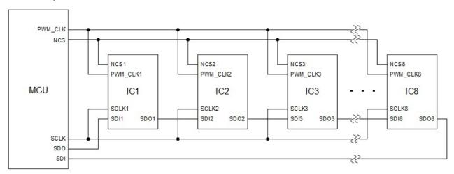
Figure 7.28 Example SPI daisy-chain connection (eight connected ICs)
