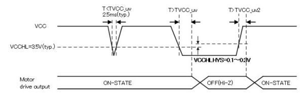
Figure 7.38 VCC under-voltage detection timing chart 1
