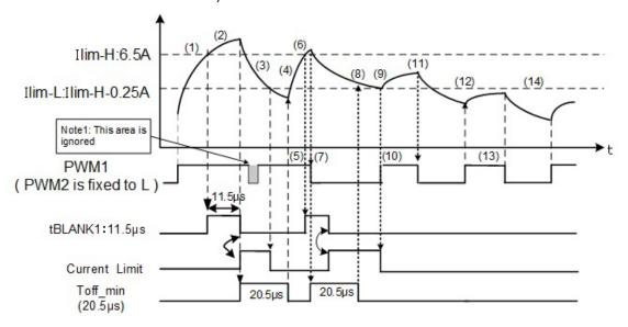
Figure 7.14 Chopper-type current-limit control
