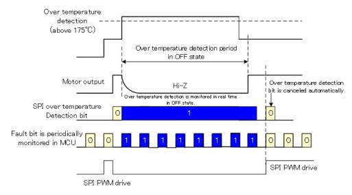
Figure 7.41 Over-temperature detection detailed timing chart
