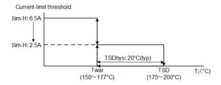
Figure 7.17 Temperature-adjusted current-limit control
