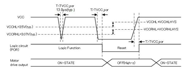
Figure 7.39 VCC under-voltage POR timing chart 1
