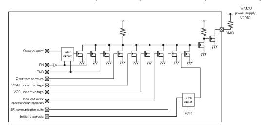
Figure 7.10. Example DIAG output circuit configuration
