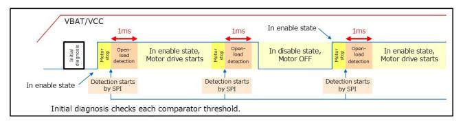
Open-load detection during non-operation: conceptual timing chart
