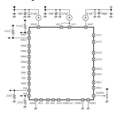
Figure 11.1. Current consumption measurement circuit diagram
