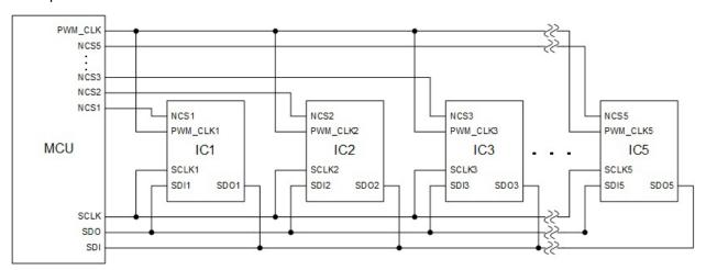
Figure 7.27 Example SPI parallel connection (five connected ICs)
