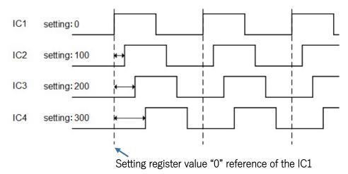
Figure 7.33 ON delay time when using multiple H-bridges
