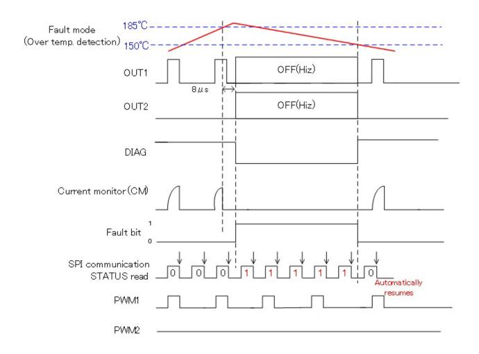
Figure 7.13 Over-temperature detection timing chart
