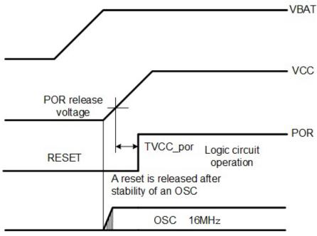
Figure 7.25 OSC circuit starting operation
