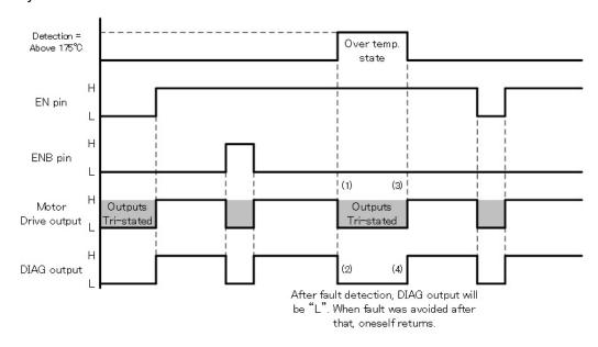
Figure 7.40 Over-temperature detection timing chart
