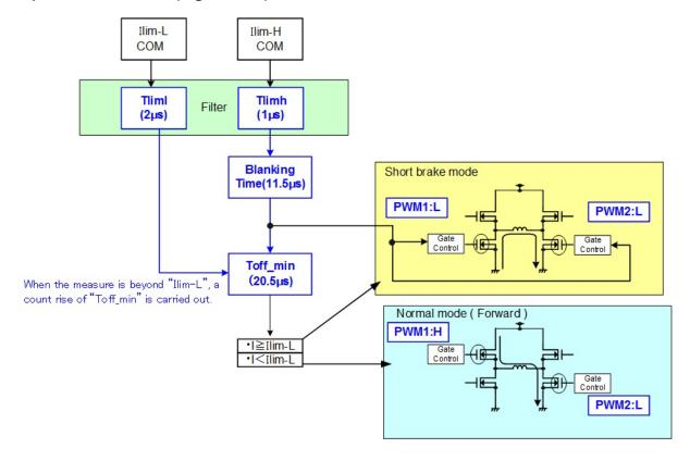
Figure 7.16 Current-limit control circuit operation flowchart
