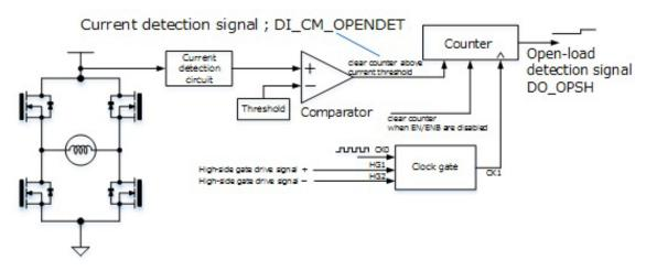
Figure 7.22 Open-load detection during operation: block diagram
