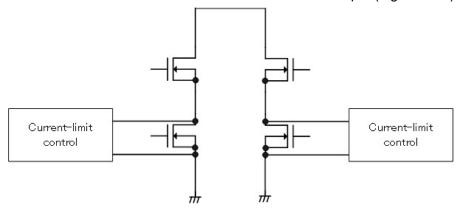
Figure 7.15 Current measurement points in current-limit control
