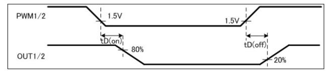
Figure 10.2. Driver output delay time
