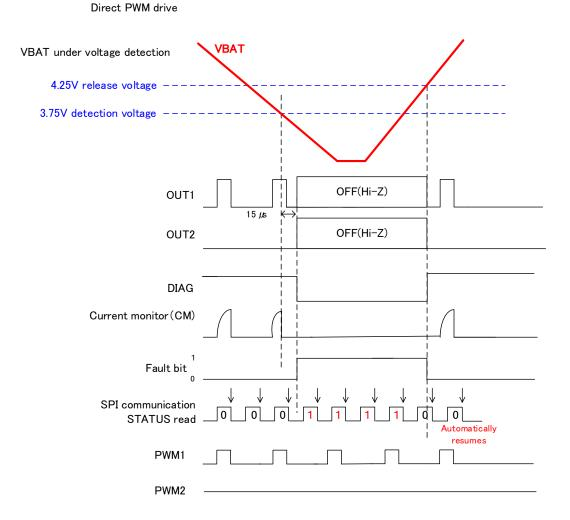
Figure 7.12. VBAT under-voltage detection timing chart
