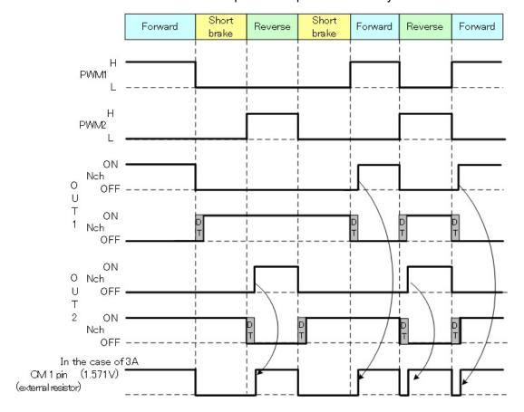
Figure 7.19 High-side current monitoring timing chart
