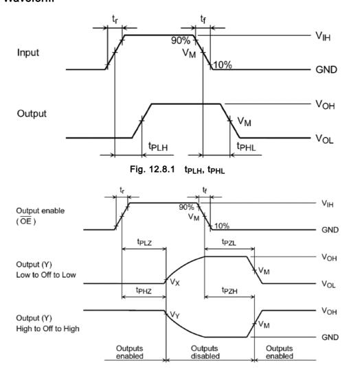
Fig. 12.8.2 t<sub>PLZ</sub>, t<sub>PHZ</sub>, t<sub>PZL</sub>, t<sub>PZH</sub>
