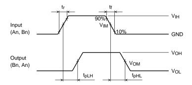
Figure 2  $t_{pLH}$ ,  $t_{pHL}$
