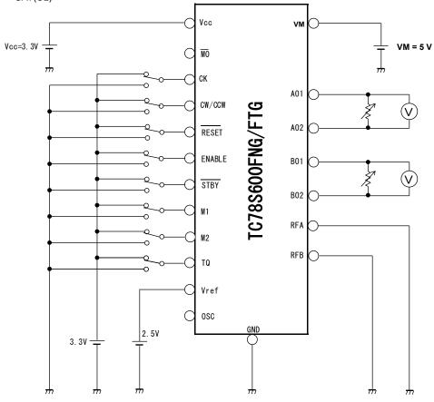
Test circuit 5:  $V_{F\,U},\,V_{F\,L}$
