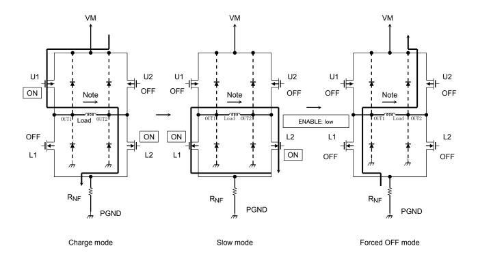
Parasitic diodes exist in the output transistors as shown above.
