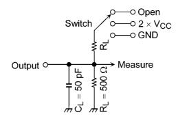
Table 11.4.1 Parameter for AC Test Circuit
