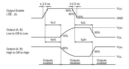
Fig. 11.5.1 AC Waveform t<sub>PLZ</sub>, t<sub>PHZ</sub>, t<sub>PZL</sub>, t<sub>PZH</sub>
