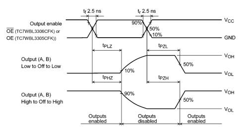
Fig. 11.6.2 AC Waveform t<sub>PLZ</sub>, t<sub>PHZ</sub>, t<sub>PZL</sub>, t<sub>PZH</sub>
