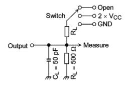
Fig. 11.6.1 AC Test Circuit
