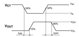
Figure 1 t<sub>r</sub>, t<sub>f</sub>, t<sub>ON</sub>, t<sub>OFF</sub> Waveforms
