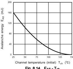
Fig. 8.14 E<sub>AS</sub> - T<sub>ch</sub> (Guaranteed Maximum)
