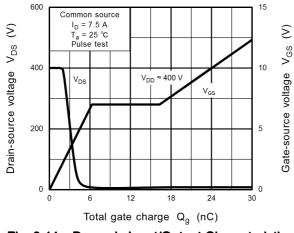
Fig. 8.11 Dynamic Input/Output Characteristics
