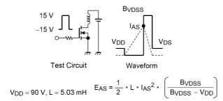
Fig. 8.16 Test Circuit/Waveform
