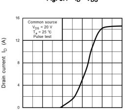
Gate-source voltage  $V_{GS}$  (V) Fig. 8.3 Ip - V<sub>GS</sub>
