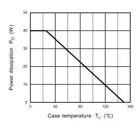
Fig. 8.15 P<sub>D</sub> - T<sub>c</sub> (Guaranteed Maximum)
