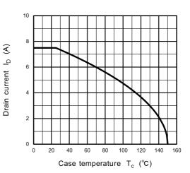
Fig. 8.12 I<sub>D</sub> - T<sub>c</sub> (Guaranteed Maximum)
