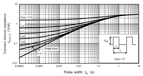
Fig. 8.13 r<sub>th</sub> - t<sub>w</sub> (Guaranteed Maximum)
