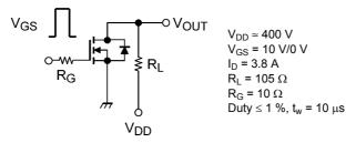
Fig. 6.2.1 Switching Time Test Circuit
