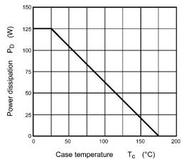
Fig. 8.11 P<sub>D</sub> - T<sub>c</sub> (Guaranteed Maximum)
