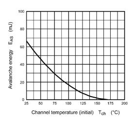
Fig. 8.14 E<sub>AS</sub> - T<sub>ch</sub> (Guaranteed Maximum)
