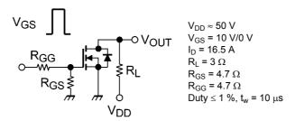
Fig. 6.2.1 Switching Time Test Circuit
