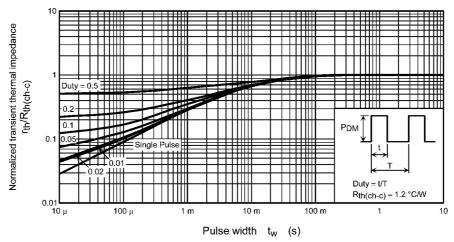
Fig. 8.12  $r_{th}/R_{th(ch-c)} - t_w$  (Guaranteed Maximum)
