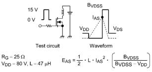
Fig. 8.15 Test Circuit/Waveform
