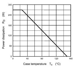
Fig. 8.15 P<sub>D</sub> - T<sub>c</sub> (Guaranteed Maximum)
