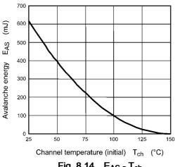
Fig. 8.14 E<sub>AS</sub> - T<sub>ch</sub> (Guaranteed Maximum)
