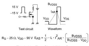
Fig. 8.16 Test Circuit/Waveform
