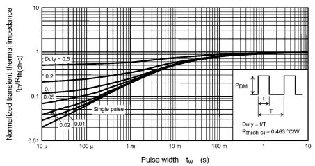
Fig. 8.13 r<sub>th</sub> - t<sub>w</sub> (Guaranteed Maximum)
