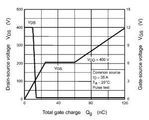
Fig. 8.12 Dynamic Input/Output Characteristics
