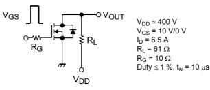
Fig. 6.2.1 Switching Time Test Circuit
