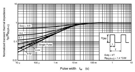
Fig. 8.12  $r_{th}/R_{th(ch-c)} - t_w$ (Guaranteed Maximum)
