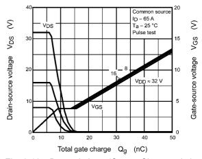
Fig. 8.10 Dynamic Input/Output Characteristics
