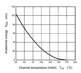
Fig. 8.14 E<sub>AS</sub> - T<sub>ch</sub> (Guaranteed Maximum)
