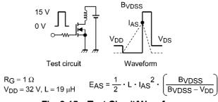
Fig. 8.15 Test Circuit/Waveform
