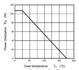
Fig. 8.11 P<sub>D</sub> - T<sub>c</sub> (Guaranteed Maximum)
