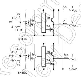
Note: A 0.1- $\mu F$  bypass capacitor must be connected between pin 8 and pin 5.
