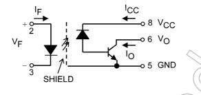
Note: A  $0.1\mu$ F bypass capacitor must be connected between pin 8 and pin 5.
