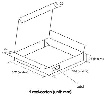
Note: Taping reel diameter:  $\phi330$  mm
