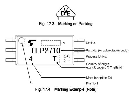
Note: The above marking is applied to the photocouplers that have been qualified according to option (D4) of EN60747.
