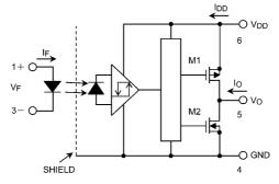
Note: A  $0.1\text{-}\mu\text{F}$  bypass capacitor must be connected between pin 6 and pin 4.
