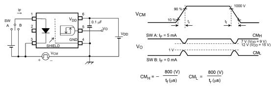
Fig. 12.1.8 Common-Mode Transient Immunity Test Circuit and Waveform
