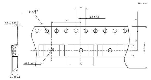
Table Tape Dimensions (unit: mm, tolerance: ±0.1)
