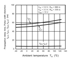
Fig. 12.2.13  $t_{pLH}$ ,  $t_{pHL}$ ,  $|t_{pHL}-t_{pLH}|$  -  $T_a$
