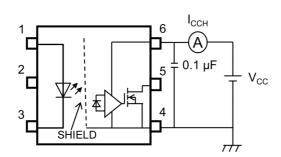
Fig. 13.1.3 I<sub>CCH</sub> Test Circuit
