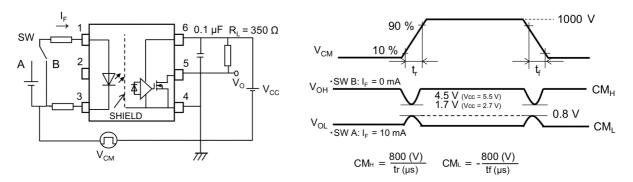
Fig. 13.1.7 Common-Mode Transient Immunity and Waveform
