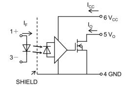
Note: A  $0.1\mbox{-}\mu\mbox{F}$  bypass capacitor must be connected between pin 6 and pin 4.
