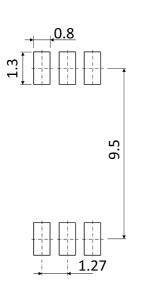
Fig. 15.1 Lead Forming Option (standard)
