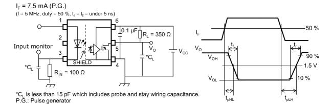
Fig. 13.1.6 Switching Time Test Circuit and Waveform
