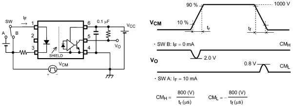
Fig. 13.1.6 Common-Mode Transient Immunity and Waveform
