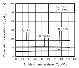
Fig. 13.2.12  $|t_{pHL} - t_{pLH}| - T_a$
