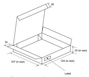
Fig. 18.4.1 1 reel/carton (unit: mm)
