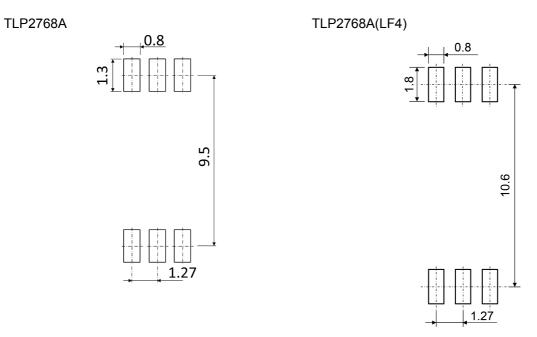
Fig. 15.1 Lead Forming Option (standard)
