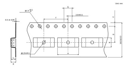
Table Tape Dimensions (unit: mm, tolerance: ±0.1)
