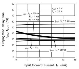
Fig. 13.2.15  $t_{pHL}$ ,  $t_{pLH}$  -  $I_F$
