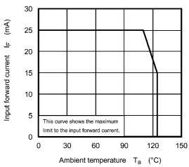
Fig. 13.2.2 I<sub>F</sub> - T<sub>a</sub>
