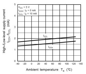
Fig. 13.2.9 I<sub>CCH</sub>, I<sub>CCL</sub> - Ta
