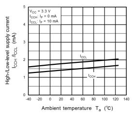
Fig. 13.2.10 I<sub>CCH</sub>, I<sub>CCL</sub> - Ta
