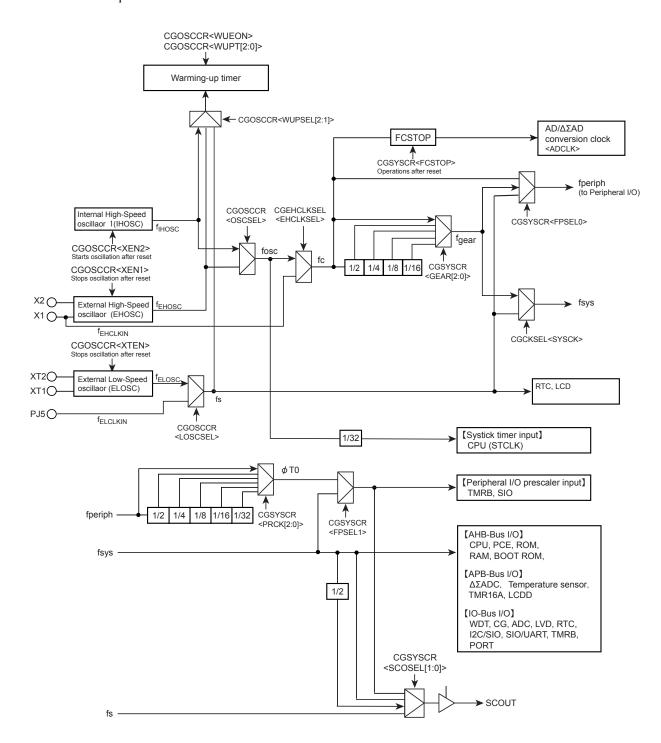
Figure 6-1 Clock Block Diagram
