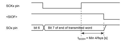
Figure 12-19 Data retention time of the last bit at the end of transmission
