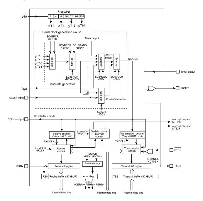
Figure 11-1 Serial Channel Block Diagram
