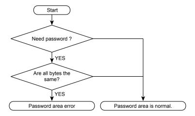
Figure 20-10 Password area check flowchart
