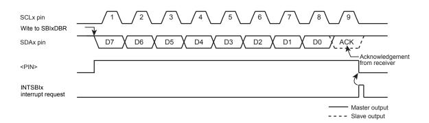
Figure 12-8 <BC[2:0]>= "000",<ACK>= "1" (Transmitter Mode)
