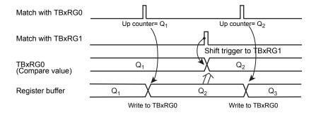
Figure 9-3 Register Buffer Operation
