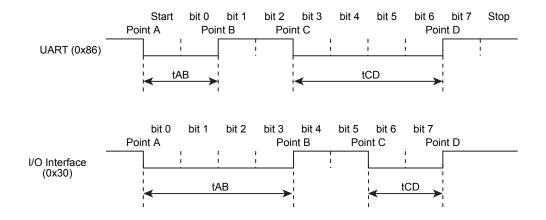
Figure 20-6 Serial operation mode determination data
