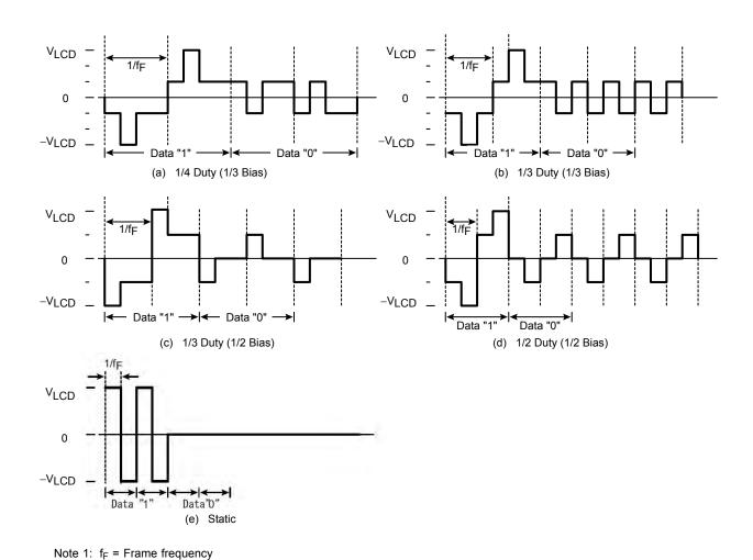
Figure 17-2 LCD Drive Waveforms (Potential Difference between COM and SEG Pins)
