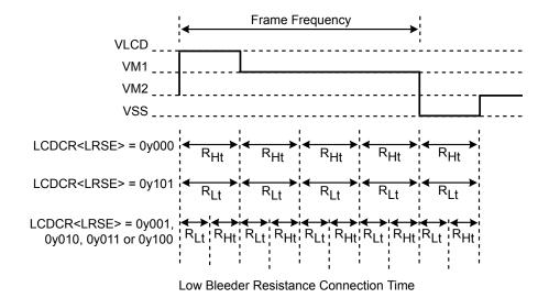
RLt: Period during which low resistance is connected (high resistance and low resistance are connected in parallel)
