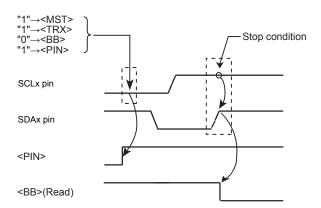
Figure 12-11 Generating the Stop Condition
