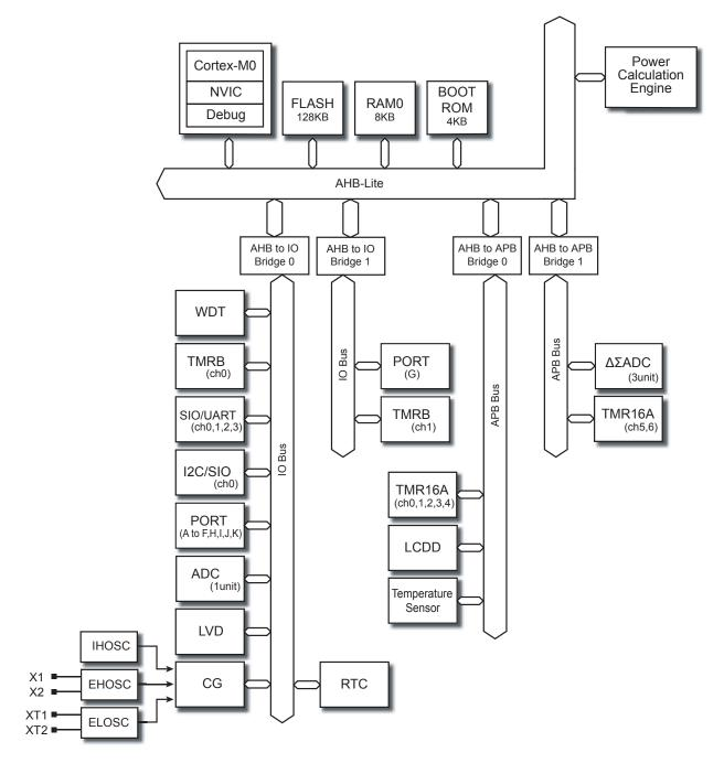
Figure 1-1 Block Diagram
