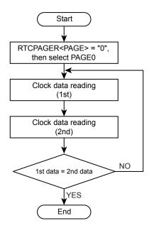
Figure 16-2 Flowchart of the clock data reading
