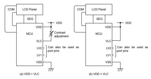
When internal bleeder resistance is used (LCDCR2<BRSEL>="1")
