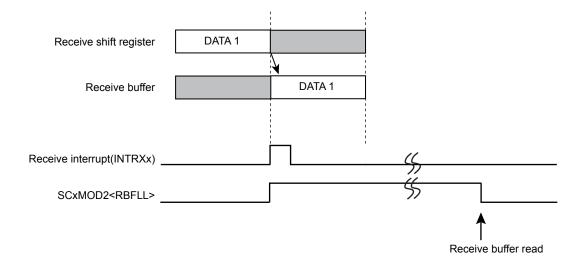
Figure 11-5 Receive Buffer Operation
