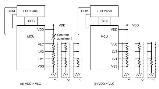
When external bleeder resistance is used (LCDCR2<BRSEL>="0")
