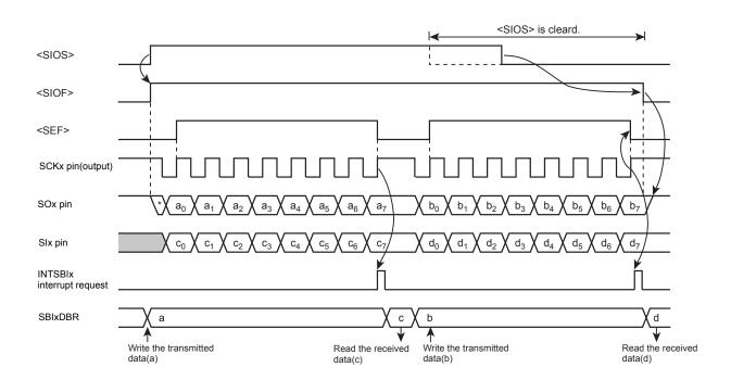
Figure 12-18 Transmit/Receive Mode (Example: Internal Clock)
