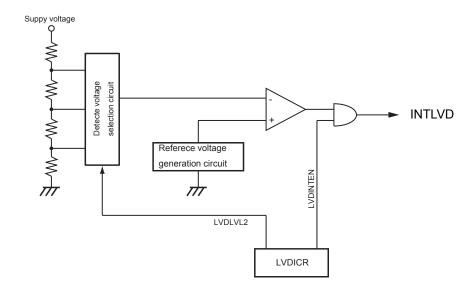
Figure 18-1 Block diagram of LVD (described only LVD interrupt circuit)
