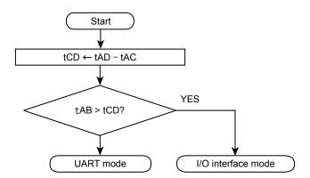
Figure 20-8 Serial operation mode determination flowchart
