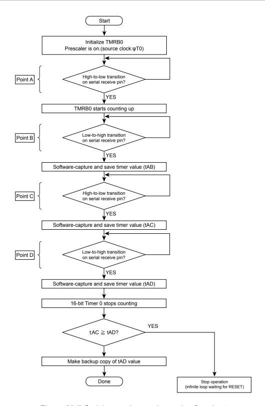
Figure 20-7 Serial operation mode receive flowchart
