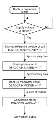
Figure 14-2 Boot-up procedure
