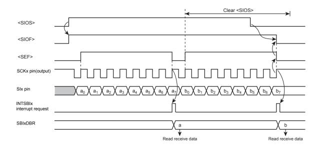
Figure 12-17 Receive Mode (Example: Internal Clock)
