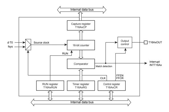
Figure 10-1 Block diagram of TMR16A
