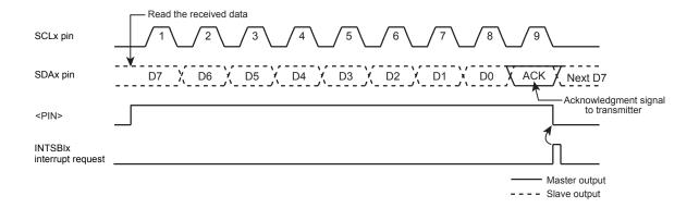
Figure 12-9 <BC[2:0]>= "000",<ACK>= "1" (Receiver Mode)
