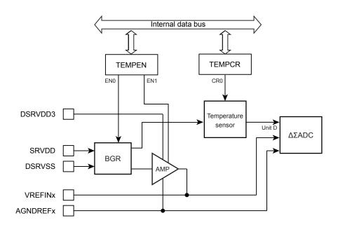
Figure 15-1 Block diagram of Temperature sensor
