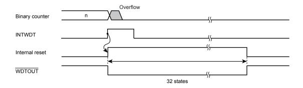
Figure 19-3 Internal reset generation
