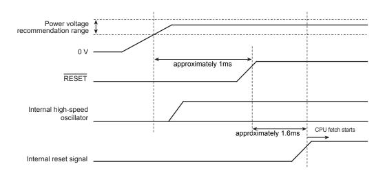
Figure 5-1 Cold Reset Operation Sequence
