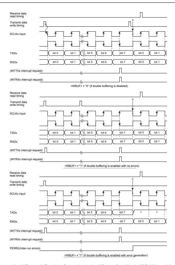
Figure 11-18 Transmit/Receive Operation in the I/O Interface Mode (SCLK Input Mode)
