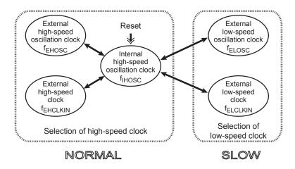
Figure 6-2 System clock switching
