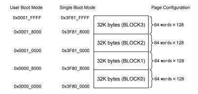
Figure 20-1 Block configuration
