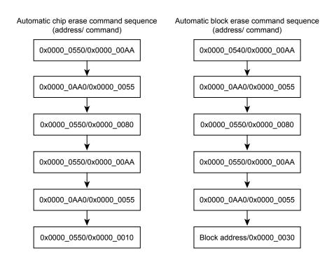
Figure 20-5 Flowchart of automatic erase
