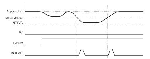
Figure 18-2 low voltage detection Timing
