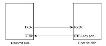
Figure 11-8 Handshake Function
