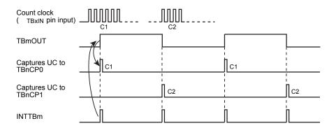
Figure 9-6 Frequency measurement
