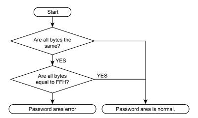
Figure 20-9 Password area check flowchart
