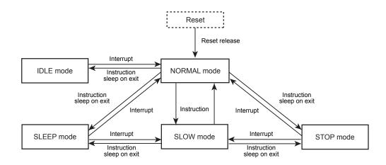
Figure 6-3 Mode Transition Diagram
