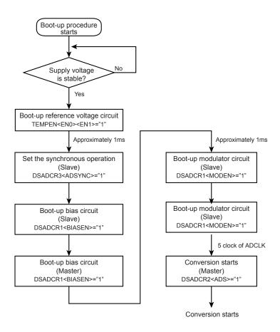
Figure 14-4 Synchronous start function procedure
