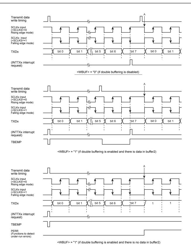
Figure 11-14 Transmit Operation in the I/O Interface Mode (SCLK Input Mode)
