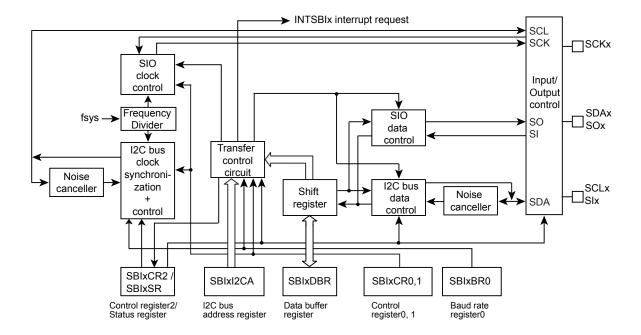
Figure 12-1 Block Diagram of Serial Bus Interface
