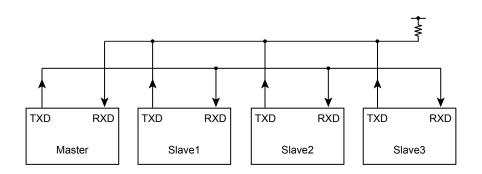
Figure 11-19 Serial Links to Use Wake-up Function
