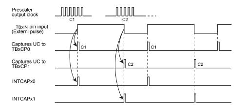
Figure 9-7 Pulse width measurement
