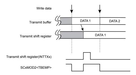
Figure 11-7 Operation of Transmission Buffer (Double-buffer is enabled)
