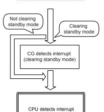
Interrupt lines used for clearing a standby mode are connected to the CPU via the clock generator.
