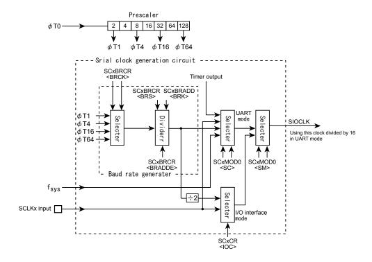
Figure 11-3 Serial clock generation circuit
