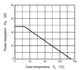
Fig. 8.12 P<sub>D</sub> - T<sub>c</sub> (Guaranteed Maximum)
