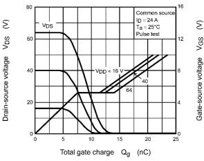
Fig. 8.10 Dynamic Input/Output Characteristics
