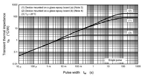
Fig. 8.13 r<sub>th</sub> - t<sub>w</sub> (Guaranteed Maximum)
