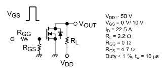
Fig. 6.2.1 Switching Time Test Circuit
