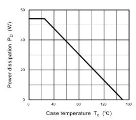
Fig. 8.15 P<sub>D</sub> - T<sub>c</sub> (Guaranteed Maximum)
