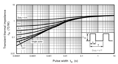
Fig. 8.13 r<sub>th</sub> - t<sub>w</sub> (Guaranteed Maximum)
