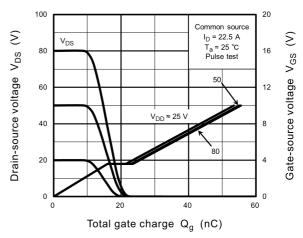
Fig. 8.10 Dynamic Input/Output Characteristics
