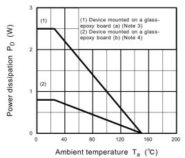
Fig. 8.14 P<sub>D</sub> - T<sub>a</sub> (Guaranteed Maximum)
