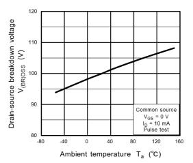
Fig. 8.7 V<sub>(BR)DSS</sub> - T<sub>a</sub>
