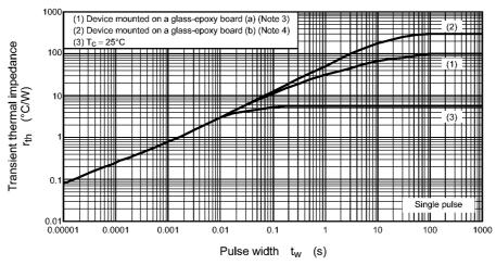
Fig. 8.13 r<sub>th</sub> - t<sub>w</sub> (Guaranteed Maximum)
