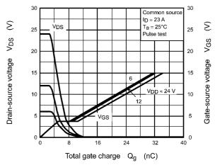
Fig. 8.10 Dynamic Input/Output Characteristics
