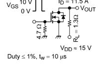
Fig. 6.2.1 Switching Time Test Circuit
