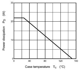
Fig. 8.12 P<sub>D</sub> - T<sub>c</sub> (Guaranteed Maximum)
