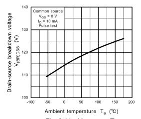
Fig. 8.11 V<sub>(BR)DSS</sub> - T<sub>a</sub>
