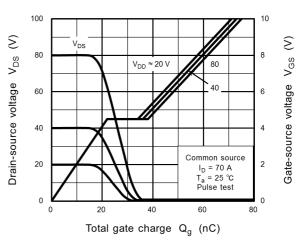
Fig. 8.14 Dynamic Input/Output Characteristics
