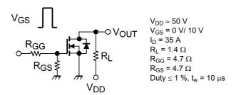
Fig. 6.2.1 Switching Time Test Circuit
