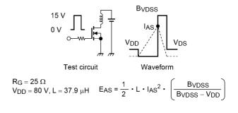
Fig. 8.16 Test Circuit/Waveform
