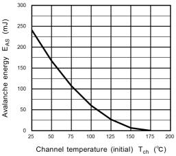
Fig. 8.15 E<sub>AS</sub> - T<sub>ch</sub>(Guaranteed Maximum)
