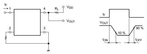
Fig. 13.1 Switching Time Test Circuit and Waveform
