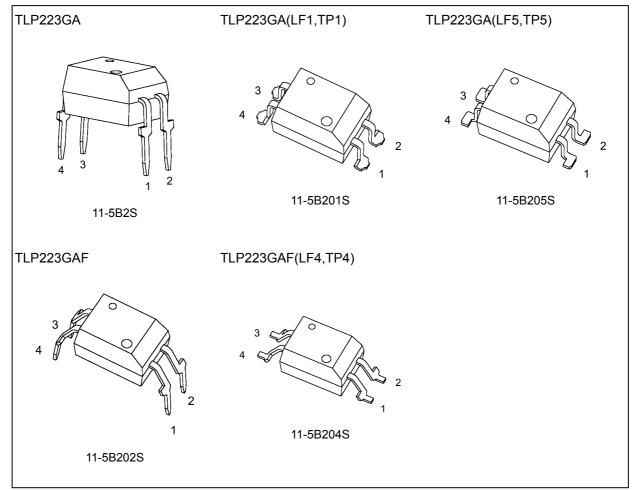
Note: Through-hole type: TLP223GA, TLP223GAF Lead forming option: (LF1), (LF4), (LF5) Taping option: (TP1), (TP4), (TP5)
