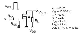
Fig. 6.2.1 Switching Time Test Circuit
