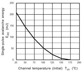
Fig. 8.15 E<sub>AS</sub> - T<sub>ch</sub>(Guaranteed Maximum)
