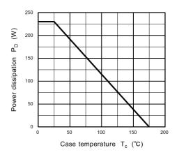
Fig. 8.19 P<sub>D</sub> - T<sub>c</sub> (Guaranteed Maximum)
