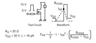
Fig. 8.16 Test Circuit/Waveform
