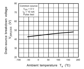
Fig. 8.11 V<sub>(BR)DSS</sub> - T<sub>a</sub>
