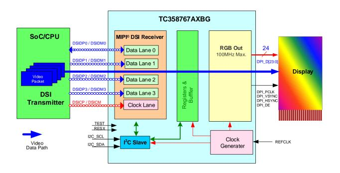
Figure 1.3 System Overview with TC358767AXBG in MODE\_S2P Configuration
