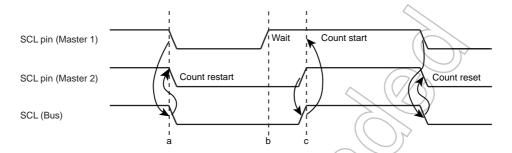
Figure 16-4 Clock Synchronization
