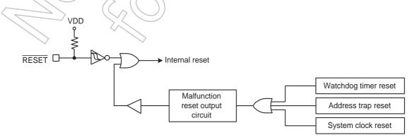
Figure 2-15 Reset Circuit
