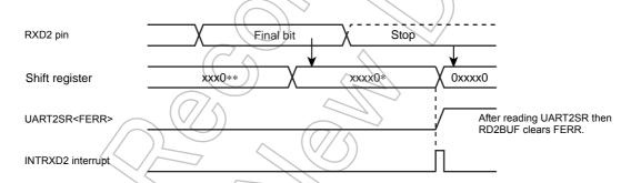
Figure 13-6 Generation of Framing Error
