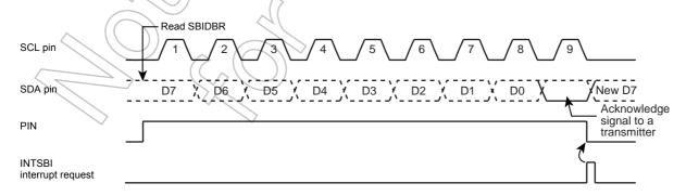
Figure 16-11 Example of when BC = "000", ACK = "1"
