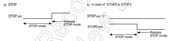
Figure 18-3 Priority of STOP pin and STOP0 to STOP3 pins
