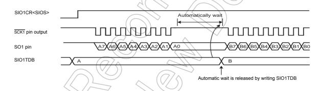
Figure 14-2 Automatic-wait Function (Example of transmit mode)
