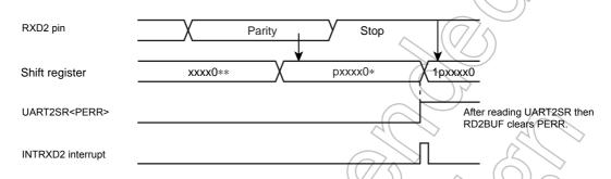
Figure 13-5 Generation of Parity Error
