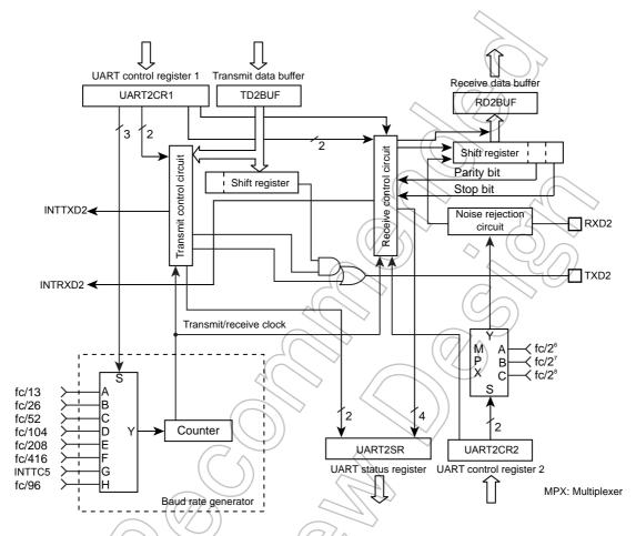
Figure 13-1 UART2 (Asynchronous Serial Interface)
