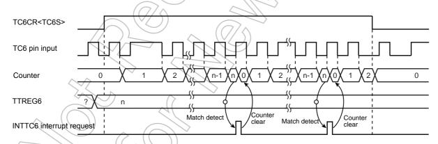
Figure 11-3 8-Bit Event Counter Mode Timing Chart (TC6)
