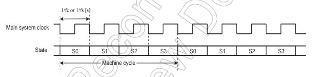
Figure 2-5 Machine Cycle
