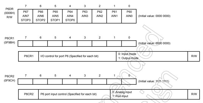
Note 1: The port placed in input mode reads the pin input state. Therefore, when the input and output modes are used together, the output latch contents for the port in input mode might be changed by executing a bit manipulation instruction.
