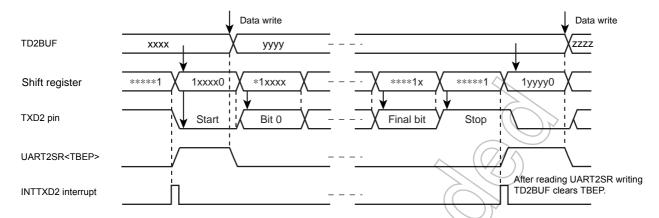
Figure 13-9 Generation of Transmit Data Buffer Empty
