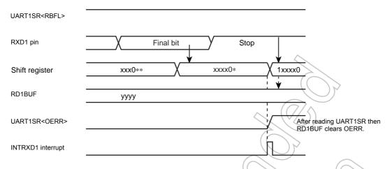
Figure 12-7 Generation of Overrun Error
