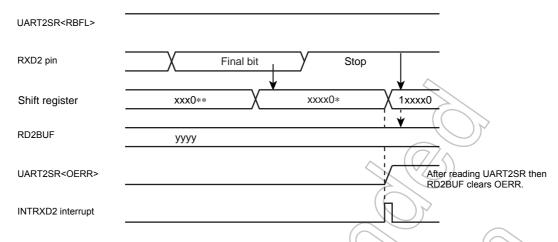
Figure 13-7 Generation of Overrun Error
