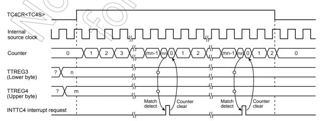
Figure 10-6 16-Bit Timer Mode Timing Chart (TC3 and TC4)
