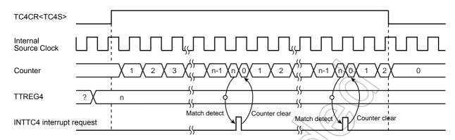
Figure 10-2 8-Bit Timer Mode Timing Chart (TC4)
