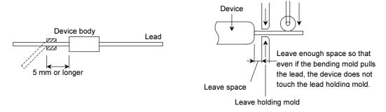
Figure 3.3 How to Bend Leads Figure 3.4 How to Bend Leads Using Metal Mold
