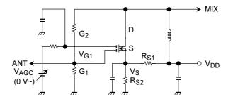
Figure 4.1 Typical AGC Circuit in a Dual-Gate MOSFET
