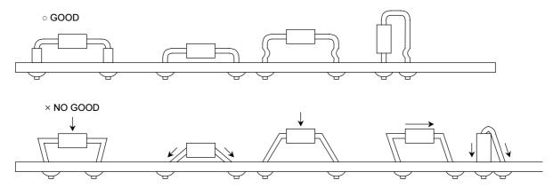
Figure 3.6 Example of Mounting on Printed-Circuit Board
