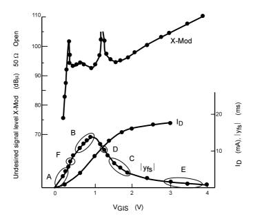
Figure 4.2 I<sub>D</sub>, |y<sub>fs</sub>|, X-Mod-V<sub>G1S</sub> Characteristics
