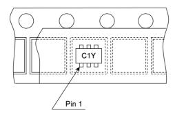
Note: TE85N is tape packing of products which are symmetrical in both their internal components and external leads, so that device orientation is unimportant.
