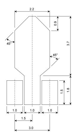
(13) 6-pin ultra-super-mini and 6-pin thin ultra-super-mini package (US6/TU6/UF6)
