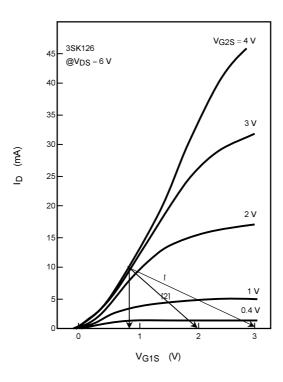
Figure 4.3 I<sub>D</sub> vs. V<sub>G1S</sub>
