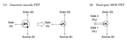
Figure 1.7 Symbols Used for Junction Cascode FET and Dual-Gate MOSFET
