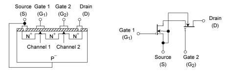
Figure 1.6 Structure and Equivalent Connection Drawings of Dual-Gate MOSFET
