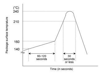
Figure 3.8 Sample Temperature Profile for Infrared or Hot Air Reflow
