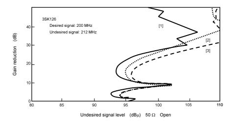
Figure 4.4 1% Cross Modulation Characteristics
