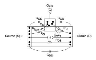
Figure 1.8 Equivalent Circuit in Relation to Structure of a FET
