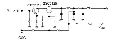
Figure 2.6 TV Tuner VHF Mixer Circuit
