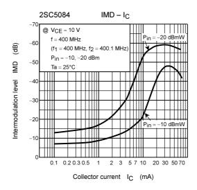
Figure 5.2 Inter-Modulation Characteristics (2SC5084)
