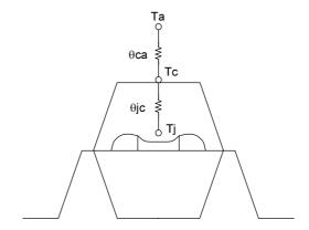
Figure 3.2 Thermal Resistance of Package
