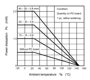
Figure 4.2 Pc (max) when Mounted on Alumi-Ceramic Board
