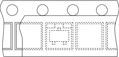
6.3.8 Tape Layout for 4-Pin Ultra-Super-Mini Package...(USQ)
