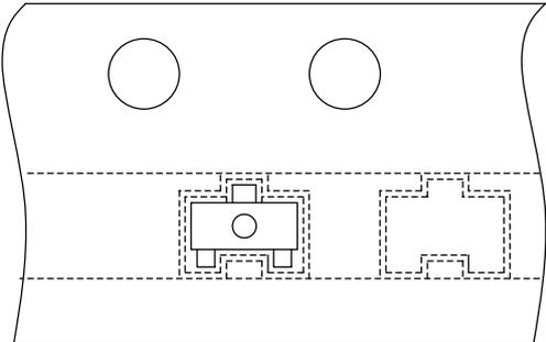
6.3.14 Tape Layout for Extreme-Super-Min Coaxial Package...(ESC)
