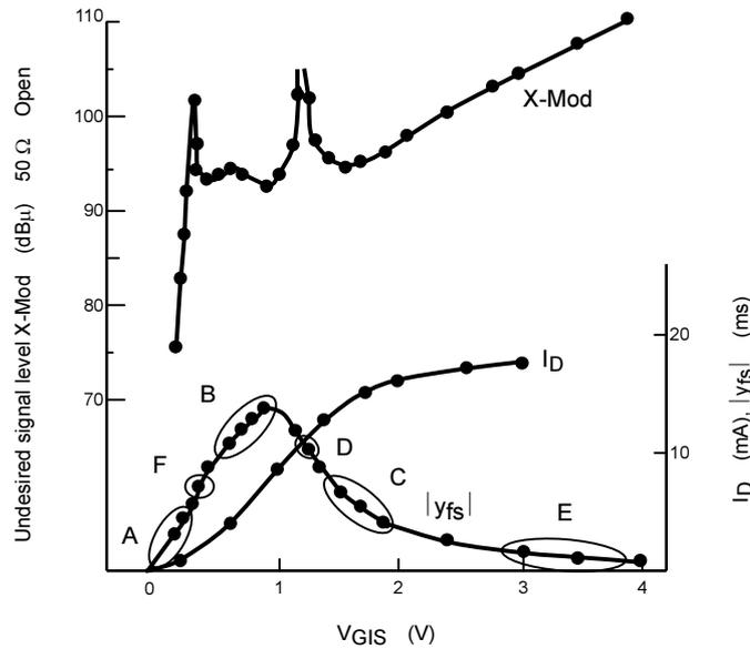
**Figure 4.2  $I_D$ ,  $|y_{fs}|$ , X-Mod- $V_{G1S}$  Characteristics**
