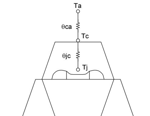
**Figure 3.2 Thermal Resistance of Package**
