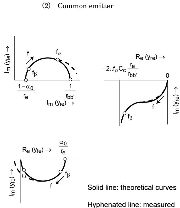
**Figure 1.14 Frequency Locus of "y" Parameters**
