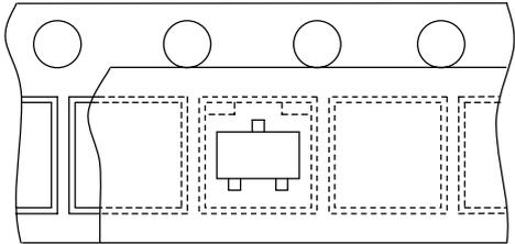
6.3.12 Tape Layout for Ultra-Super-Mini Coaxial Package...(USC)
