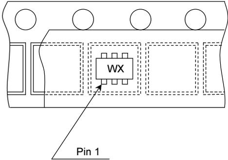
6.3.11 Tape Layout for Small-Super-Mini Package...(SSM)
