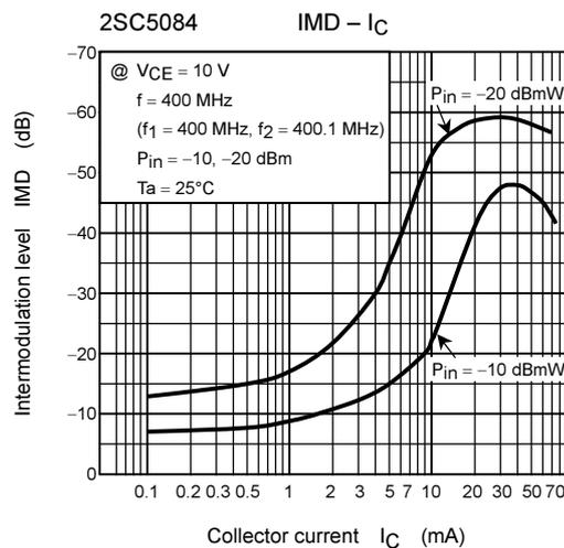
**Figure 5.2 Inter-Modulation Characteristics (2SC5084)**
