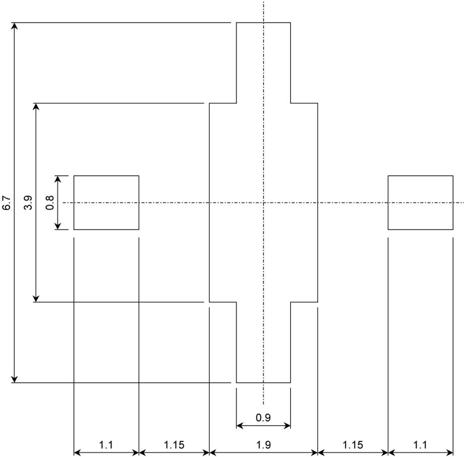
The following shows reference pad dimensions when a device mounted on a board.
