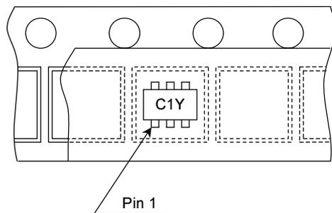
Note: TE85N is tape packing of products which are symmetrical in both their internal components and external leads, so that device orientation is unimportant.
