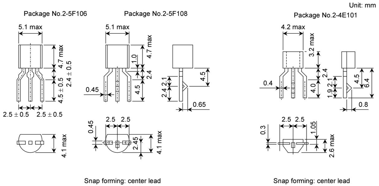
**Figure 6.1 Lead-Formed TO-92 Transistor Package Dimensions**
