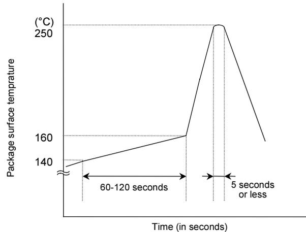
**Figure 3.9 Sample Temperature Profile for Solder Flow**
