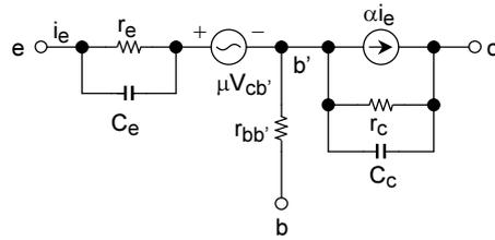
**Figure 1.1 Early's T-Type Equivalent Circuit**
