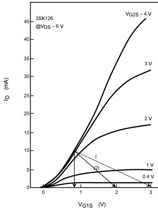
**Figure 4.3  $I_D$  vs.  $V_{G1S}$**
