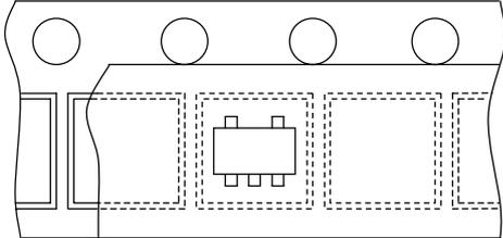
**6.3.4 Tape Layout for 6-Pin Super-Mini Package...(SM6) (SSOP6-P-0.95)**
