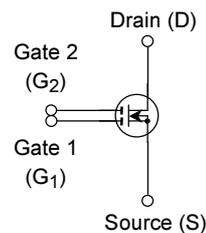
**Figure 1.7 Symbols Used for Junction Cascode FET and Dual-Gate MOSFET**
