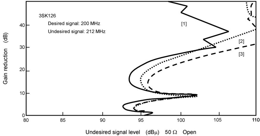
**Figure 4.4 1% Cross Modulation Characteristics**
