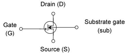
\*: The substrate gate is usually connected to the source.
