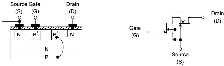
**Figure 1.5 Structure and Equivalent Connection Drawing of Cascode FET**
