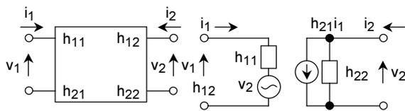
$$\begin{pmatrix} v_1 \\ i_2 \end{pmatrix} = \begin{pmatrix} h_{11} & h_{12} \\ h_{21} & h_{22} \end{pmatrix} \begin{pmatrix} i_1 \\ v_2 \end{pmatrix} = \begin{pmatrix} h_i & h_r \\ h_f & h_o \end{pmatrix} \begin{pmatrix} i_1 \\ v_2 \end{pmatrix}$$
