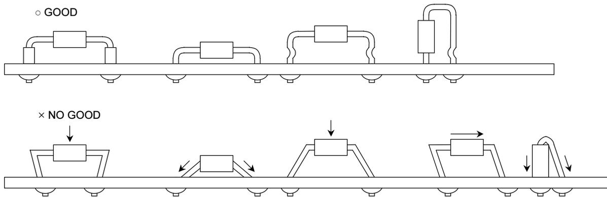
Figure 3.6 Example of Mounting on Printed-Circuit Board
