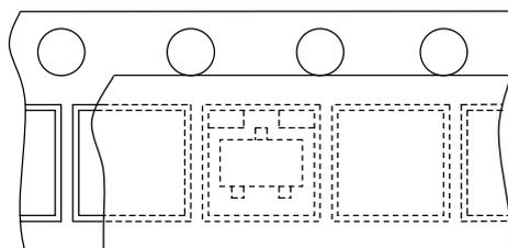
6.3.2 Tape Layout for 4-Pin Super-Mini Package...(SMQ)
