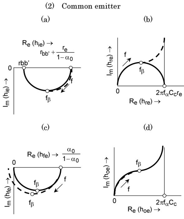
**Figure 1.13 Frequency Locus of "h" Parameters**
