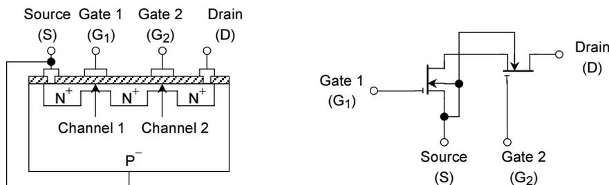
**Figure 1.6 Structure and Equivalent Connection Drawings of Dual-Gate MOSFET**
