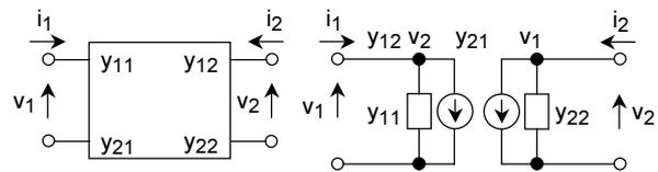
$$\begin{pmatrix} i_1 \\ i_2 \end{pmatrix} = \begin{pmatrix} y_{11} & y_{12} \\ y_{21} & y_{22} \end{pmatrix} \begin{pmatrix} v_1 \\ v_2 \end{pmatrix} = \begin{pmatrix} y_i & y_r \\ y_f & y_o \end{pmatrix} \begin{pmatrix} v_1 \\ v_2 \end{pmatrix}$$
