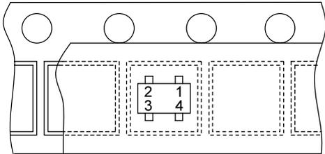
**6.3.3 Tape Layout for 5-Pin Super-Mini Package...(SMV) (SSOP5-P-0.95)**
