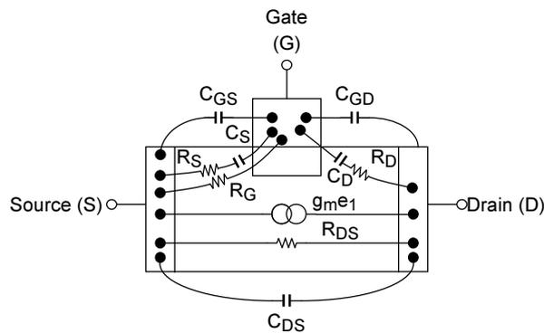
**Figure 1.8 Equivalent Circuit in Relation to Structure of a FET**
