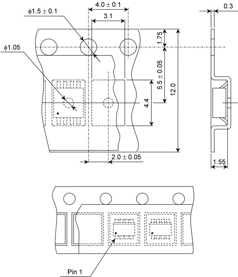
6.3.18 Tape Layout for PW-X Package...(PW-X)
