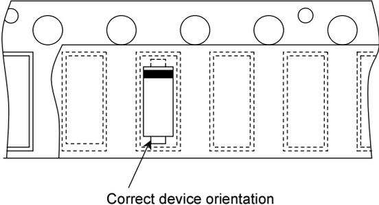
**6.3.13 Tape Layout for Extremely Thin Super-Mini Package...(TESM)**
