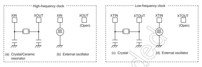
Figure 2-3 Examples of Resonator Connection
