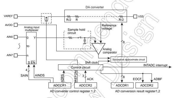
Figure 11-1 8-bit AD Converter (ADC)
