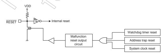
Figure 2-15 Reset Circuit
