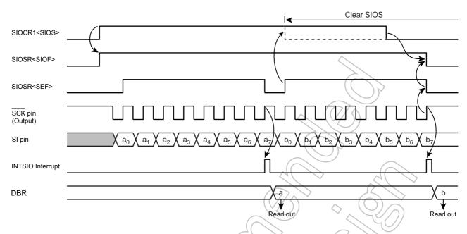
Figure 10-10 Receive Mode (Example: 8bit, 1word transfer, Internal clock)
