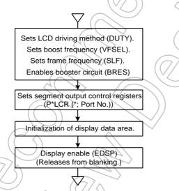
Figure 13-5 Initial Setting of LCD Driver
