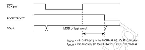
Figure 10-9 Transmiiied Data Hold Time at End of Transfer
