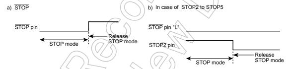
Figure 12-3 Priority of STOP pin and STOP2 to STOP5 pins
