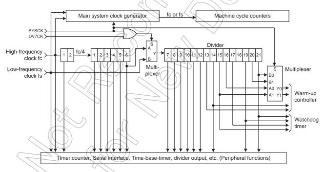
Figure 2-4 Configuration of Timing Generator
