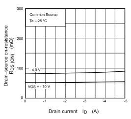
Fig. 7.4  $R_{DS(ON)}$  -  $I_D$
