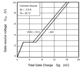
Fig. 7.11 Dynamic Input Characteristics
