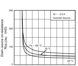
Gate–source voltage V<sub>GS</sub> (V) Fig. 7.3 R<sub>DS(ON)</sub> - V<sub>GS</sub>
