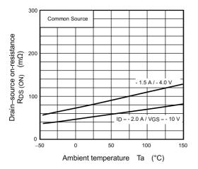
Fig. 7.5 R<sub>DS(ON)</sub> - T<sub>a</sub>
