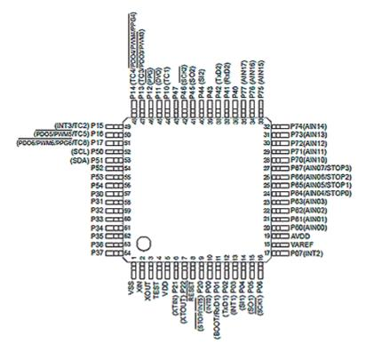
Package UG: LQFP64 ( $10 \times 10 \text{ mm}$ ) FG: QFP64 ( $14 \times 14 \text{ mm}$ )
