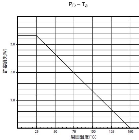
基板実装時 (140 mm × 70 mm × 1.6 mm, Cu : 50%)  $R_{th(j-a)}$  = 38°C/W
