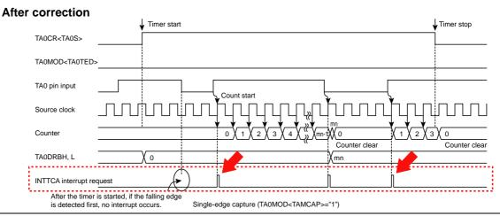
2. The timing diagram for double-edge capture indicates that no interrupt request occurs at the count start edge after the timer is started. This should be corrected so that an interrupt request occurs at the count start edge, as shown below.
