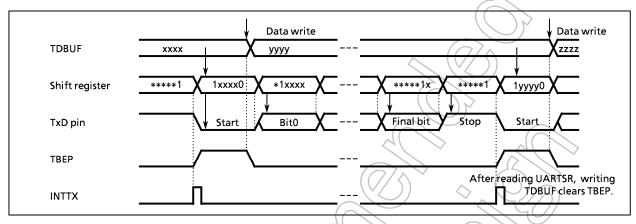
Figure 2-65. Generation of Transmit Buffer Empty
