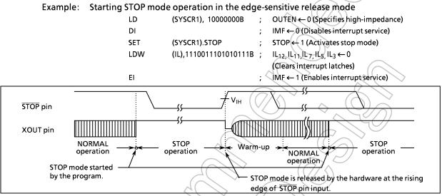
Figure 1-17. Edge-sensitive Release Mode
