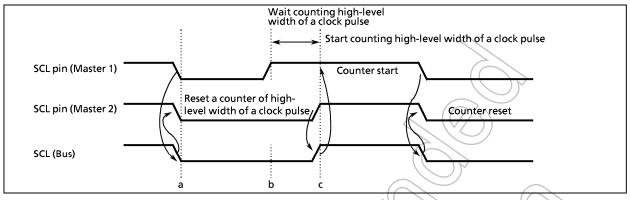
Figure 2-37. Clock Synchronization
