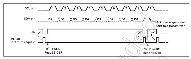
Figure 2-45. Termination of Data Transfer in Master Receiver Mode
