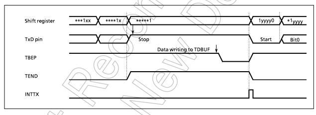
Figure 2-66. Generation of Transmit Buffer Empty
