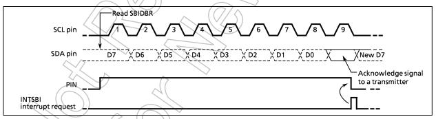
Figure 2-44. Example of when BC = "000", ACK = "1" in Receiver Mode
