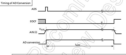
Note 1: During AD conversion, make the level of  $V_{AIN}$  stable. Note 2: i = 17 to 10, 07 to 00
