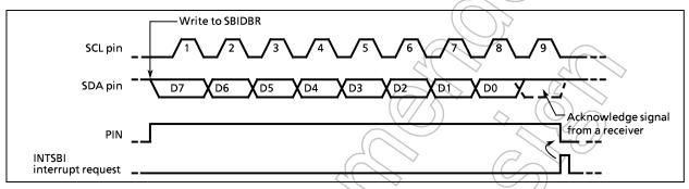
Figure 2-43. Example when BC = "000", ACK = "1" in Transmitter Mode
