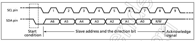
Figure 2-38. Start Condition Generation and Slave Address Generation
