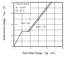
Fig. 7.2.11 Dynamic Input Characteristics
