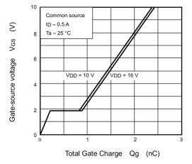
Fig. 7.1.11 Dynamic Input Characteristics
